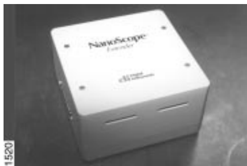
Figure 13.2. Extender™ Electronics Module (required for MFM phase detection and frequency modulation).
