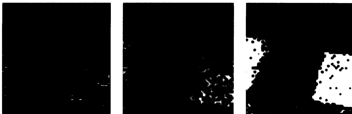
Fig. 36. Three force-slices at a distance of 300, 350, and 440 nm from the deflection of maximum load on a FITC deposit on silicon. The lighter parts of the image indicate the larger value of deflection. In each force-slice the tip is still adhering to silicon (black points), while it is already detached from the FITC deposit (white points). The number of points on FITC at which the tip is already detached increases with the distance (adapted from [231]).
